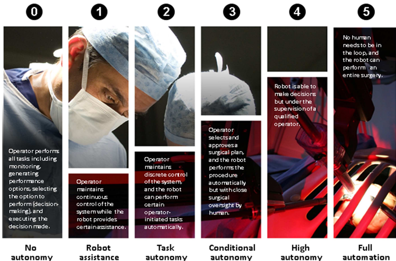
Fig. 1. Different levels of autonomy as mapped to robotic surgery. It is possible that technology may advance faster than regulatory, ethical, and legal frameworks. Risk management during implementation is critical to avoid backlash that would impede progress.
