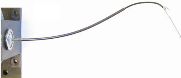
Fig. 7. Prototype steerable needle grasping a 4-0 suture needle.
