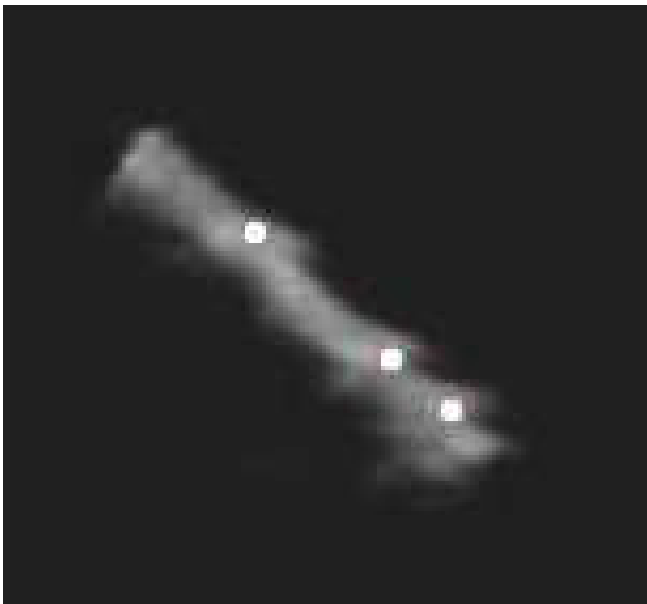
Fig. 4. 3D ultrasound image of a surgical instrument in a water tank. The results of the passive marker tracking is indicated by the white dots.
