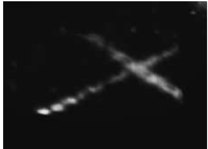
Fig. 5. 3D ultrasound image of the target X . The target was composed of two intersecting strands of nylon. This fiducial was designed to be attached to surgical targets, such as a patch.
