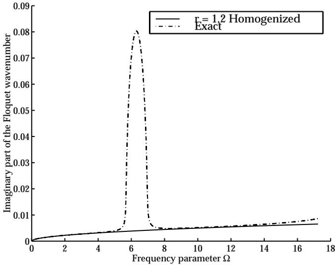
Figure 5. Imaginary part of the propagating Floquet wavenumber for a structure with two arrays having spacings  $d_1 = 1\text{m}$  and  $d_2 = 2\text{m}$ .
