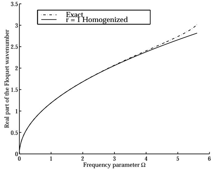
Figure 2. Real part of the propagating Floquet wavenumber for a structure with one array having a spacing  $d_1 = 1$  m.
