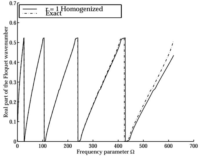
Figure 6. Real part of the propagating Floquet wavenumber for a structure with three arrays having spacings  $d_1 = 1\text{m}$ ,  $d_2 = 6\text{m}$ , and  $d_3 = 12\text{m}$ .
