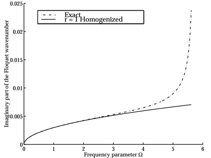
Figure 3. Imaginary part of the propagating Floquet wavenumber for a structure with one array having a spacing  $d_1 = 1$  m.
