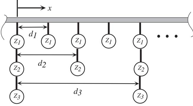
Figure 1. Thin elastic plate with three arrays of line attachments. The circles represent line impedances that extend along the  $y$  coordinate (into page).
