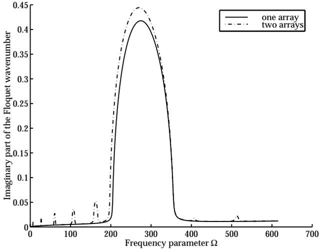
Figure 8. Imaginary part of the propagating Floquet wave in a plate with one ( $d_2 = 6$ ) and two arrays of line attachments ( $d_1 = 1$  and  $d_2 = 6$ ). The one-array case corresponds to the large spacing limit.
