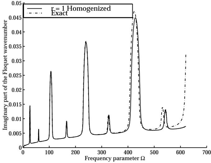
Figure 7. Imaginary part of the propagating Floquet wavenumber for a structure with three arrays having spacings  $d_1 = 1\text{m}$ ,  $d_2 = 6\text{m}$ , and  $d_3 = 12\text{m}$ .
