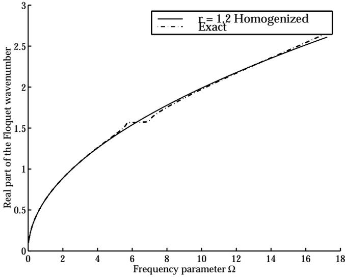
Figure 4. Real part of the propagating Floquet wavenumber for a structure with two arrays having spacings  $d_1 = 1\text{m}$  and  $d_2 = 2\text{m}$ .
