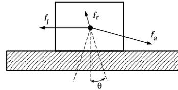
Figure 1: Block sliding to right on horizontal surface. Moment associated with friction force is neglected.
