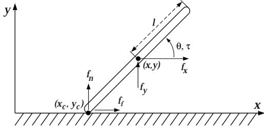
Figure 4: Planar rod of mass  $m$  and moment of inertia  $J$  in contact with immobile wall.
