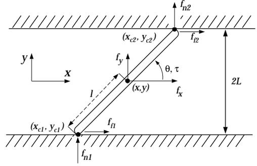
Figure 5: Planar rod of mass  $m$  and moment of inertia  $J$  in contact with two immobile walls.
