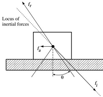
Figure 2: Block sliding to right on horizontal surface which accelerates upward.
