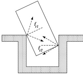
Figure 3: Wedging during peg insertion. Overlapping friction cones at contacts represent sets of possible reaction forces,  $f_{r1}$  and  $f_{r2}$ .
