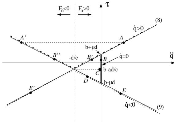
Figure 3: Scalar Case of  $\tau$  Versus  $\ddot{q}$  for  $\mu > a/c$ . In this case, there can be multiple solutions or none.
