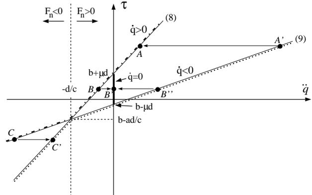
Figure 2: Scalar Case of  $\tau$  Versus  $\ddot{q}$  for  $\mu < a/c$  and  $d > 0$ . The upper, dot-dashed V corresponds to  $\dot{q} > 0$ . The lower, dotted V corresponds to  $\dot{q} < 0$ . The dark line segment on the  $\tau$ -axis is the static region where  $\dot{q} = 0$ . The horizontal arrows indicate discontinuities in acceleration which occur when  $\dot{q} = 0$ .
