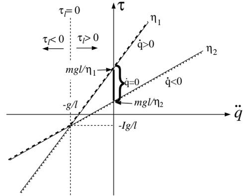
Figure 6: Graph of  $\tau$  Versus  $\ddot{q}$  for an Overhauling Screw. Since  $\alpha > \rho$ , a positive torque is required to maintain  $\dot{q} = 0$ .
