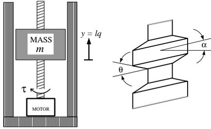
Figure 5: Screw-driven Mass. The motor applies torque  $\tau$  to the screw. The mass,  $m$ , is attached to the nut. Its displacement,  $y$ , is related to the screw displacement,  $q$ , by the screw lead,  $l$ . The helix angle,  $\alpha$  and thread angle,  $\theta$ , are also shown.
