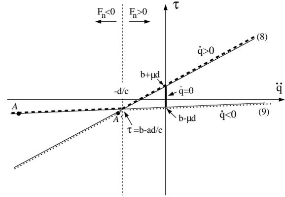
Figure 4: Near-critical Case of  $\tau$  Versus  $\ddot{q}$ . Here, the line of (9) is nearly horizontal. For  $\dot{q} > 0$ , applying  $\tau < (b - ad/c)$  moves the system to a point such as  $A$  producing a very large negative acceleration.
