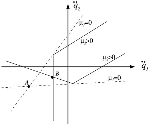
Figure 1: Constraint Equations in Acceleration Space. The frictionless solution corresponds to the intersection of the two dashed lines, point A. For  $\mu_i > 0$ , the V-shaped constraint equations intersect at B yielding a unique solution. By reorienting the V's and changing their included angles, cases of zero and multiple intersection points can be obtained.
