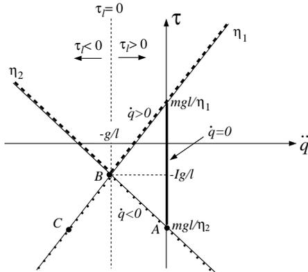
Figure 7: Graph of  $\tau$  Versus  $\ddot{q}$  for a Screw with  $(I + ml^2/\eta_2) < 0$ .
